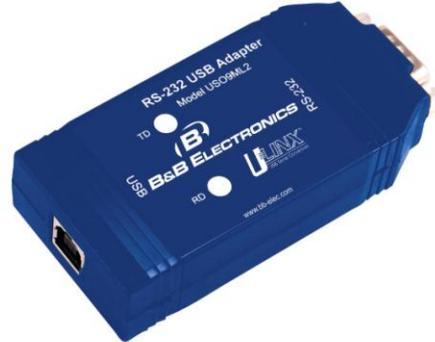
This compact, isolated USB to RS-232 converter allows you to add an RS-232 port to your USB only PC. Built to rugged specifications with two kilovolts of isolation, it will protect your PC from hazardous ground loops. The compact size makes it perfect for field service use but it is also great for instrumentation and laboratory applications. Full speed (12 Mbps) USB 2.0 support allows connectivity with modern computer technology.
